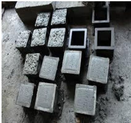
Fig 5: casting of mortar cubes
