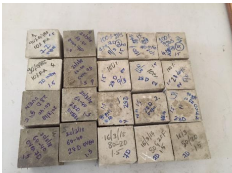
Fig 6: Demoulded mortar cubes
