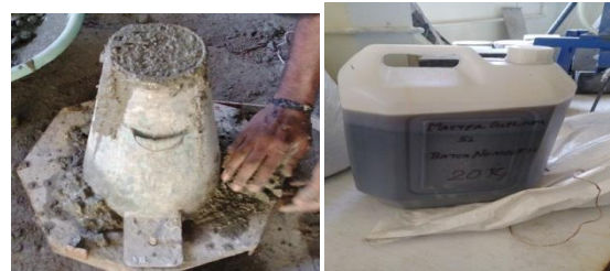
Pic 2 Slump test and glenium
