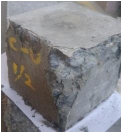
Pic 3- Cube after failure
