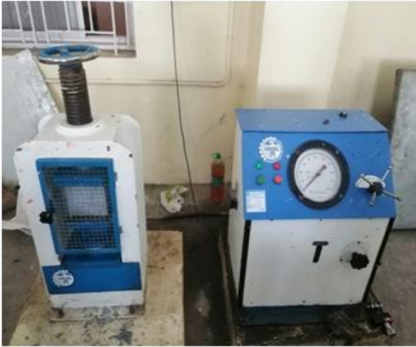
Fig. 2. Compressive strength test setup
