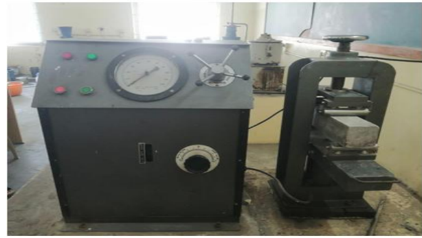
Fig. 4. Flexural strength test setup
