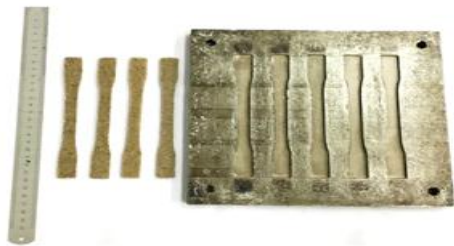
Fig. 1 Photo of molding fabrication of tensile specimens
