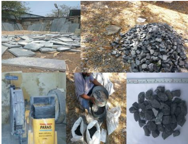
Figure1. Preparation of cuddapah waste aggregate
