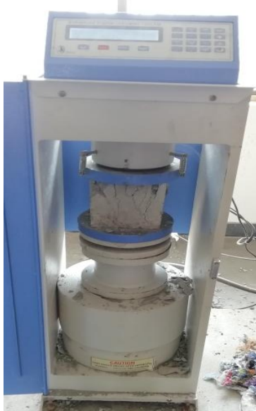
Fig.1: Testing of cube specimen
