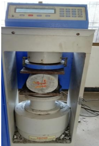
Fig.2: Test on cylindrical specimen
