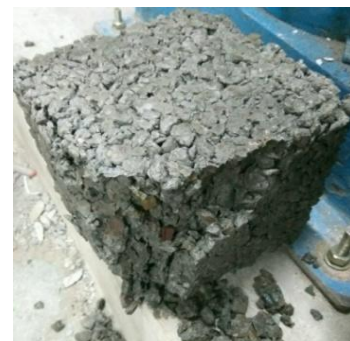
Fig. 5. Specimen containing no fibre
