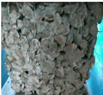
Fig. 7. Specimen containing steel fibre
