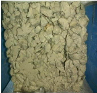
Fig. 6. Specimen containing glass fibre
