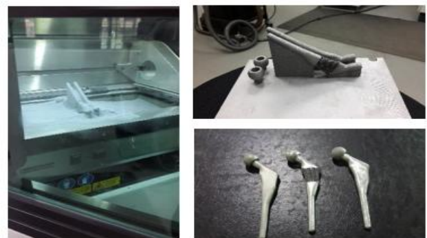
Fig. 3. Fabrication of hip implant using direct laser metal sintering.
