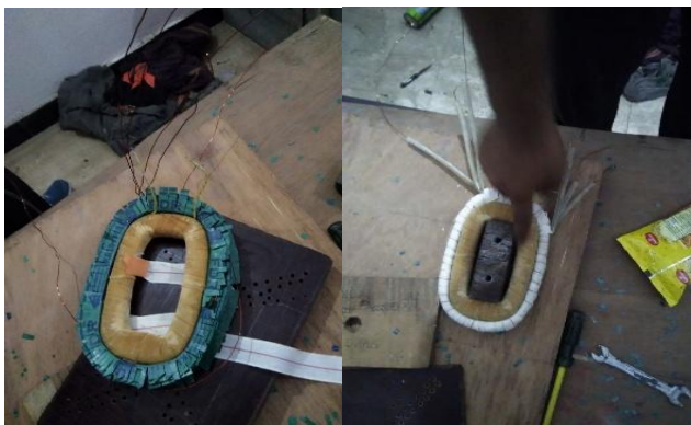
Fig. 4. Addition of Compensating winding to Field Winding
