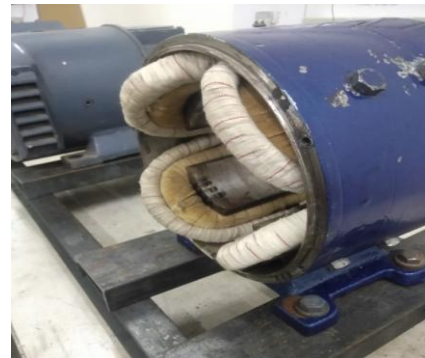
Fig. 5. Alternator with stationary field and compensating windings
