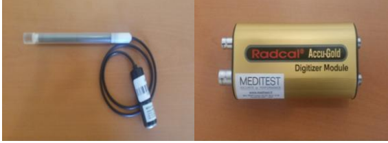
Figure 1. The ion chamber for CTDI: Radcal 10x6-3CT.
