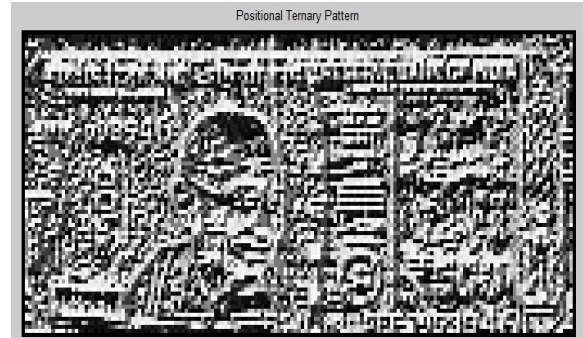
Figure. 5(d) Positional Ternary Pattern to describe edges
