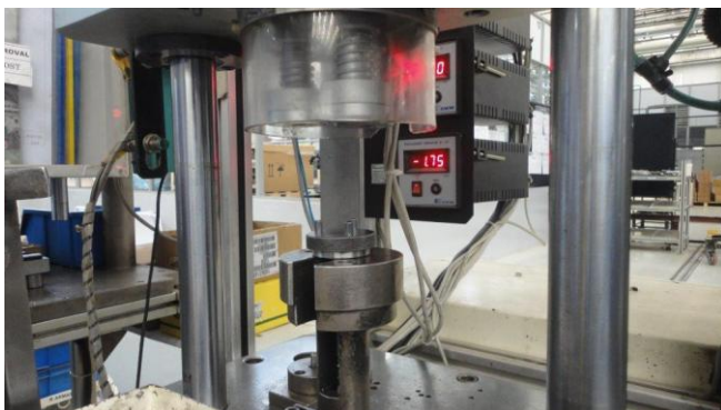
Fig.12. Load monitoring and LVDT display
