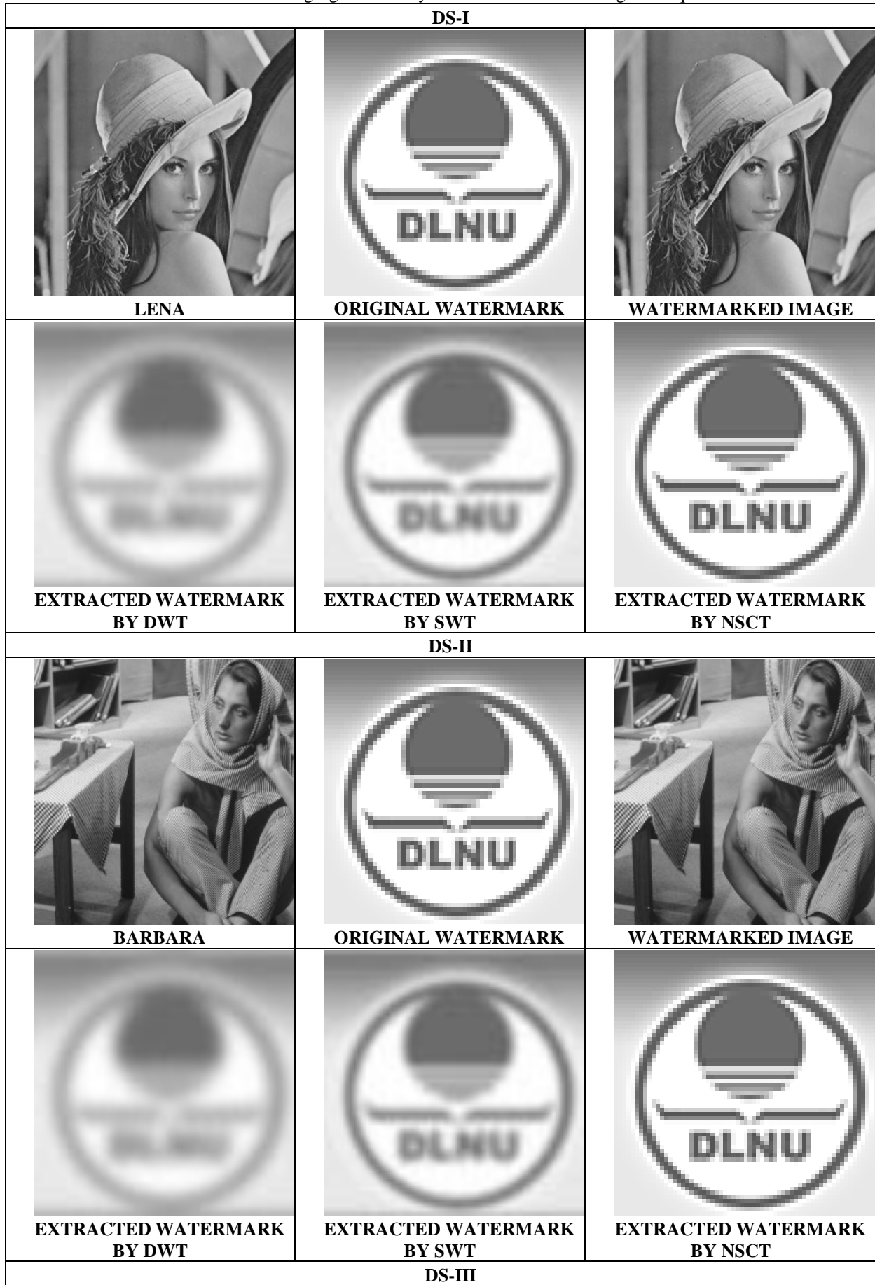
Fig. 3 shows the recovered watermark image generated by different watermarking techniques for dataset DS.
