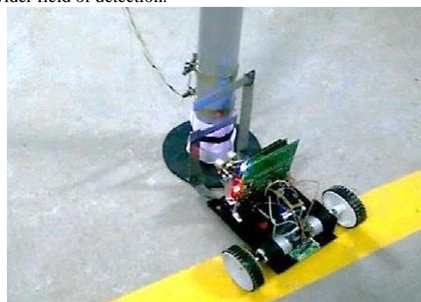
Fig.4(c). Robot docking for recharging
