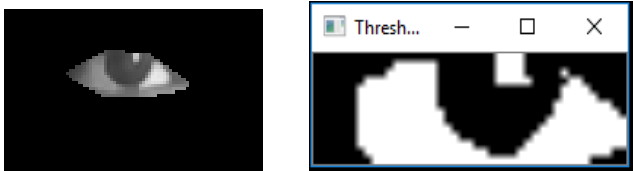
Fig. 11. Eye ball detection (a) Left eye (b) After applying threshold
