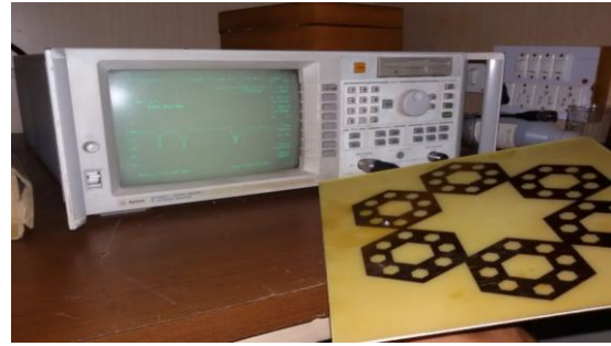
Fig.24: Experimental set up with Vector Network Analyzer (VAN)
