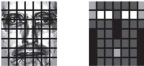
Fig2: (a) Dividing the image to 7x7 equally size cell, (b) weighting schemes after encoding the histogram for each of the cells [6]
