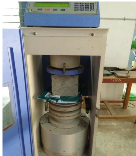
Fig. 4. Testing of Cube Specimen
