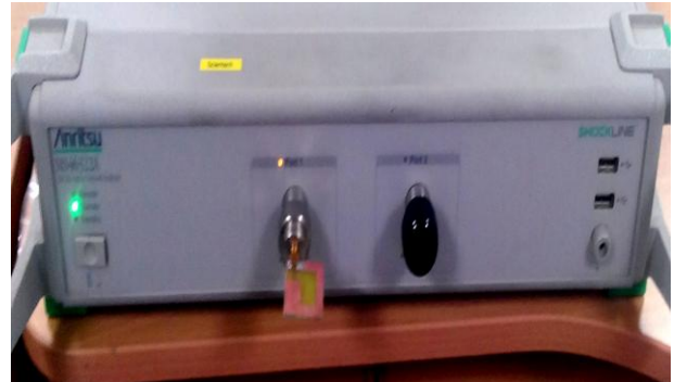
Fig. 6. Measurement of prototype performance with MS46322A vector network analyzer
