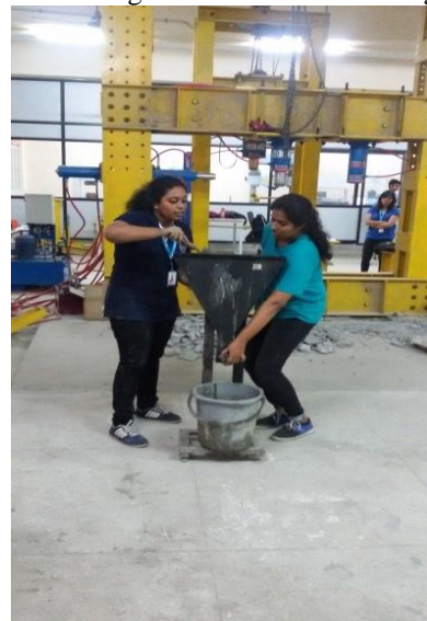
Fig. 7. Experimentation in V-Funnel Test
