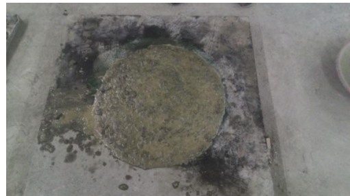
Fig. 6. Spread of SCC in the .J-Ring test
