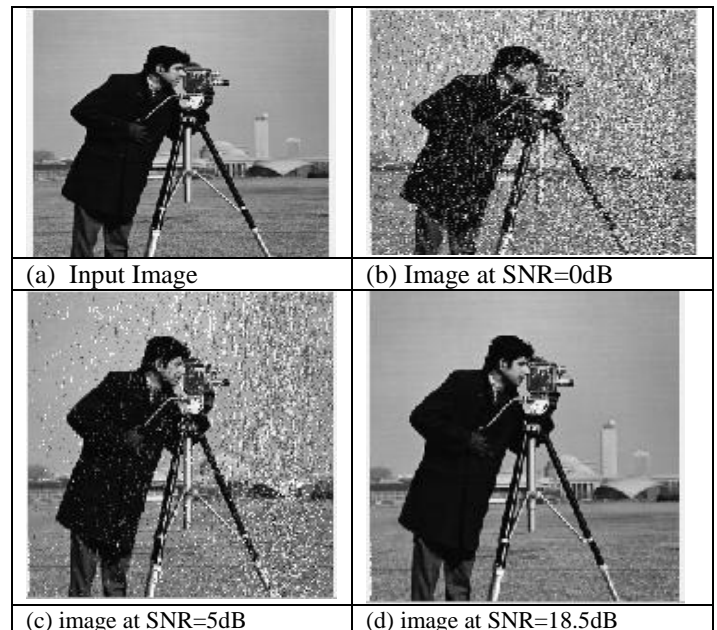
Fig.9: input image at different SNR with fading [AWGN and Rayleigh Channel]
