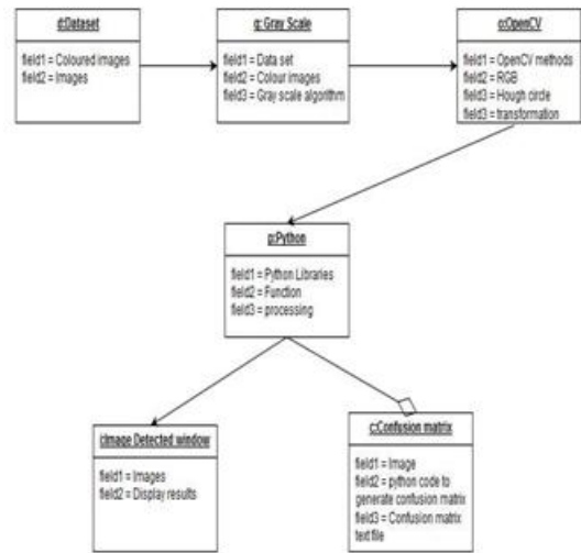
3.4: Figure.3.4:: Object diagram for fuel adulteration detection using image processing
