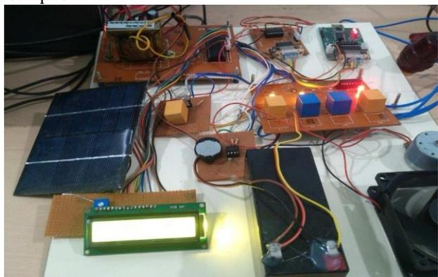
**Fig. 10 AC or Heavy devices are controlled by ZigBee during Peak time**
