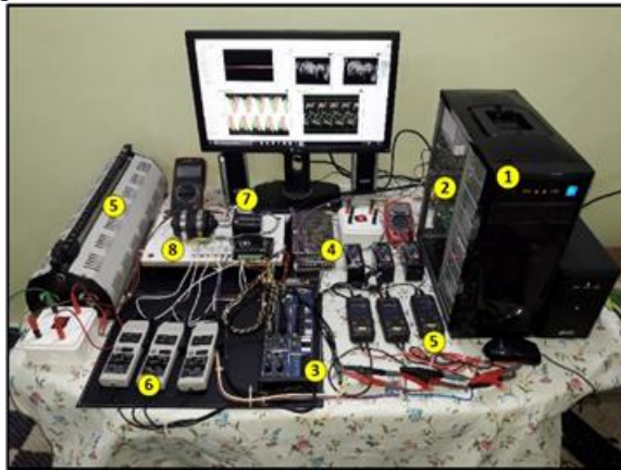
(1) Personal computer. (2) DAQ Data acquisition card. (3) BNC connectors for I/O connections. (4) Power supply. (5) High voltage differential isolating probes. (6) Oscilloscope AC/DC clamp current probe. (7) Brushless DC motor. (8) DC generator. (9) Rheostat variable resistor.
