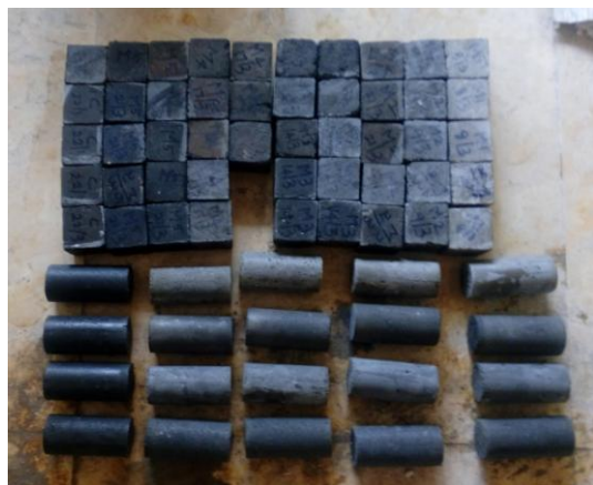
Fig.2. Specimens after casting
