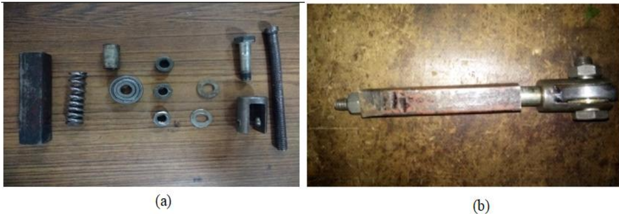
Figure 1(a) Components of burnishing tool (b) Congregated view of burnishing tool
