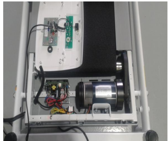
Figure 4 Conveyor drive system by PMDC motor
