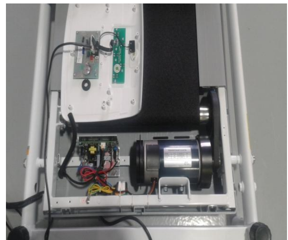
Figure 4 Conveyor drive system by PMDC motor
