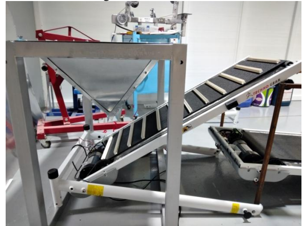
Figure 3 Hopper and conveyor units
