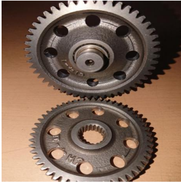
Fig. 25 Gear – 1 & 2: After Machining Implementation of scenario 1 for both
