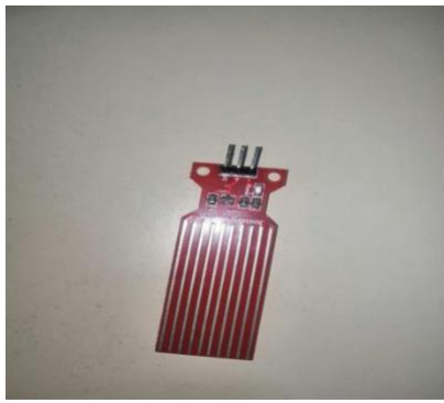
Fig.4.Water sensor for sweat detection.
