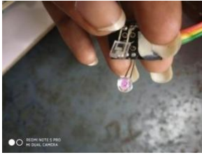
Fig.3.Pulse sensor for heart rate detection.
