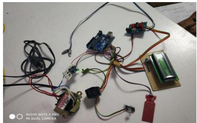
Fig.2. Stress meter using Pulse sensor and Sweat sensor.
