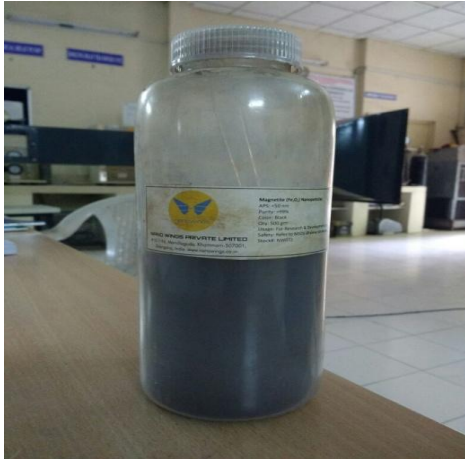
Fig 2: Magnetite ( Fe_3O_4 ) nano particles of <50nm diameter
