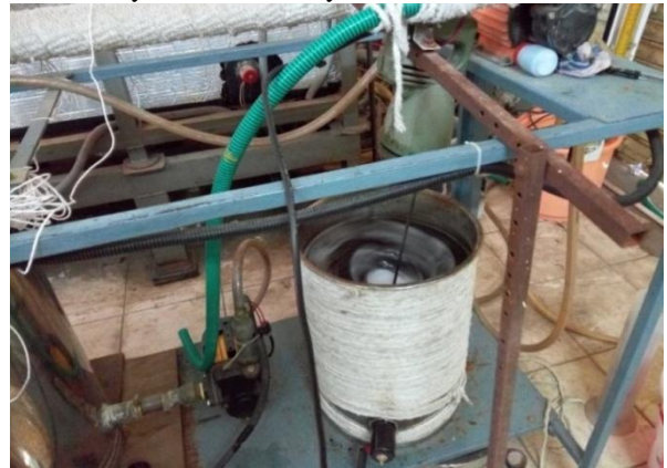
Fig 3: Nanofluid Preparation using Mechanical Stirrer
