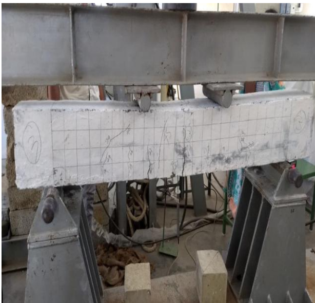
Fig: Crack Pattern of Beam (P1)
