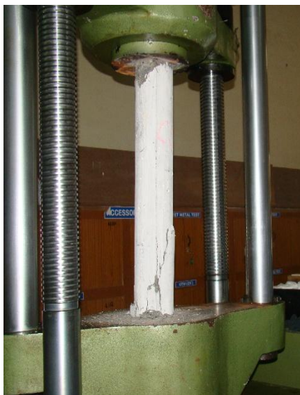
Fig. 6. Failure of Column Specimen
