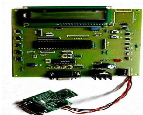
Fig. 3: Server Pi-node interfaced with ZigBee
