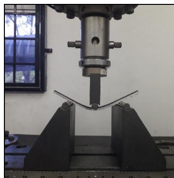
Fig 4. Specimen Set Up of Flexural Test
