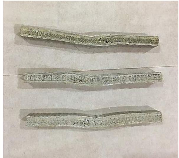
Fig. 5: Side view of the specimens under flexural load
