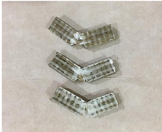
Fig. 7: Side view of the specimens after undergoing SENB test
