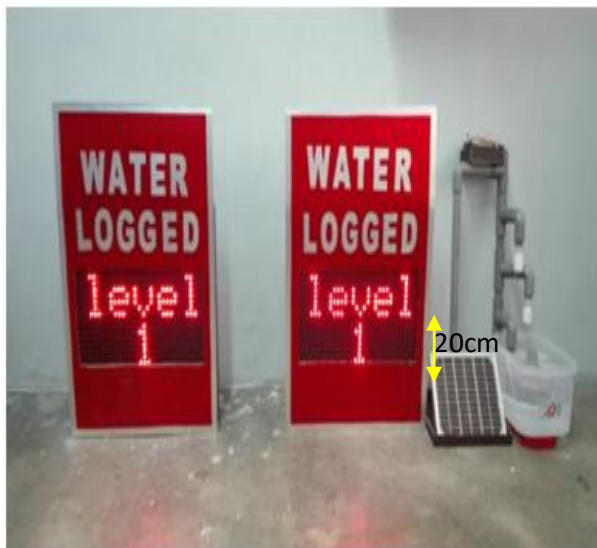
Fig. 9 When water depth is at first level
