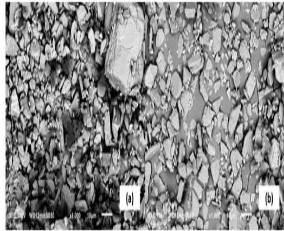
Fig. 1 Morphology of limestone – Al 2 O 3 with (a) No Acid (b) 2 ml Oxalic acid
