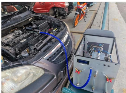
Fig. 8 The PorFC connected to a return type fuel system vehicle (Naza Citra)
