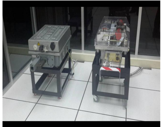
Fig. 8 Point machine Siemen SIMAX S700KM and Thales L826H
