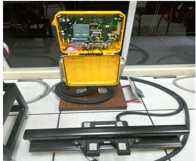
Fig. 9 Thales Axle counter with sweeper
