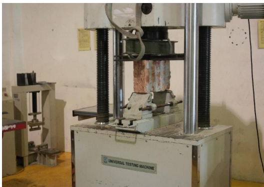
Fig. 2 Setting up for prism flexural test
