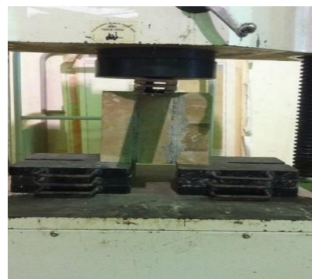
Fig. 1 Setting up for masonry shear test
