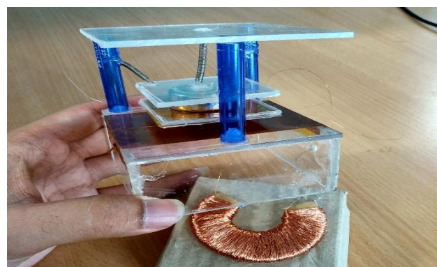
Fig. 4 Coil turns in 'O' shape
