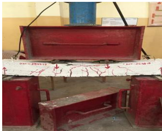
Fig 9: Cracking Pattern of C + 20% FA + 3% FrA Sample
