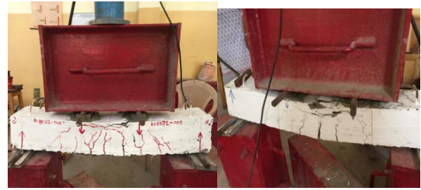
Fig.11. Cracking Pattern of C + 30% FA + 3% FrA Sample
