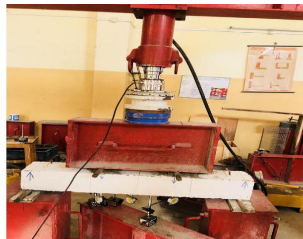
Fig.7. Placing of Beam
