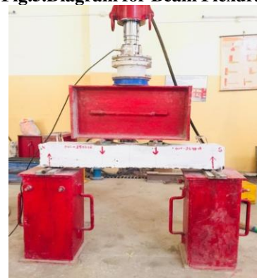
Fig.6. Setup for Flexural Test
