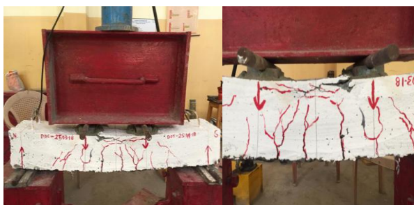
Fig: 10 Cracking Pattern of C + 20% FA + 3% FrA Sample
