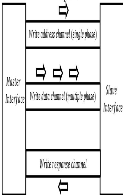
Figure 2. Write Architecture
