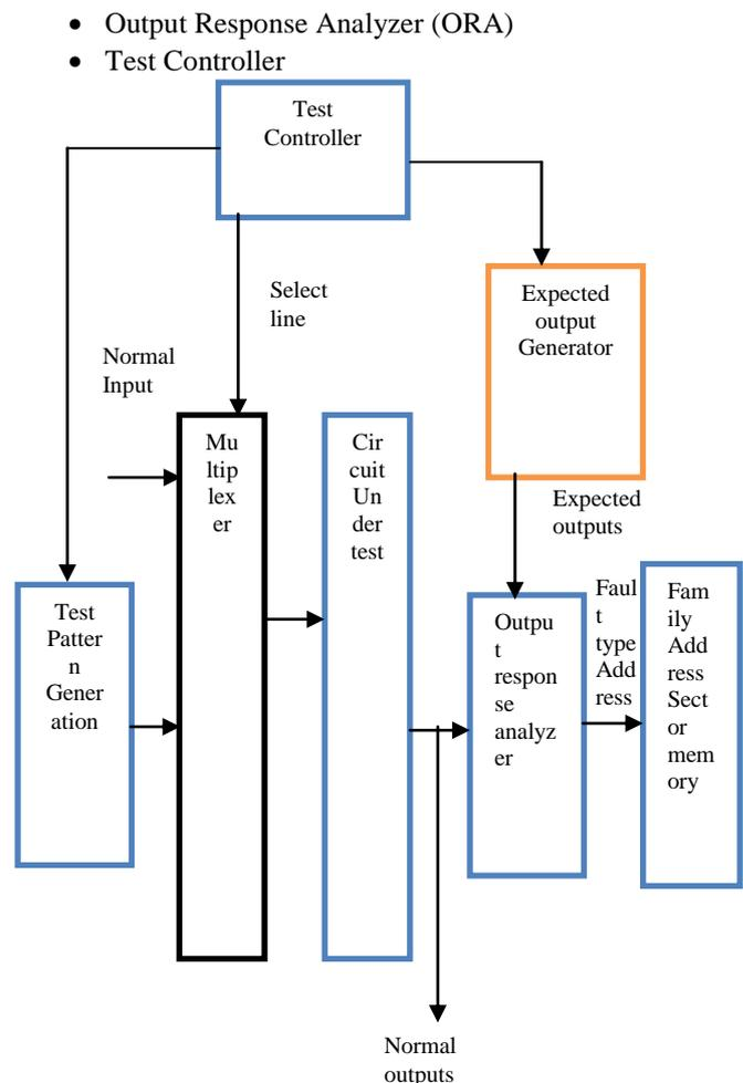
Figure 1: Conventional BIST Block Diagram
