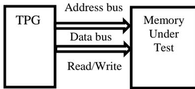
Figure 5: General scheme for testing Memory [4].
