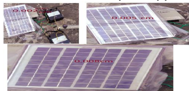
Fig. 3. Experimental set-up with different thickness of plastic.
