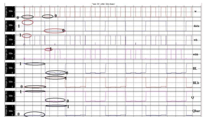
Fig. 4. Writing information into 8T traditional CNTFET Static-RAM Structure.
