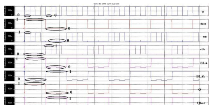
Fig. 6. Writing data into Dual-Port 8T CNTFET SRAM Cell Structure using bit lines (BLA & BLAb).
