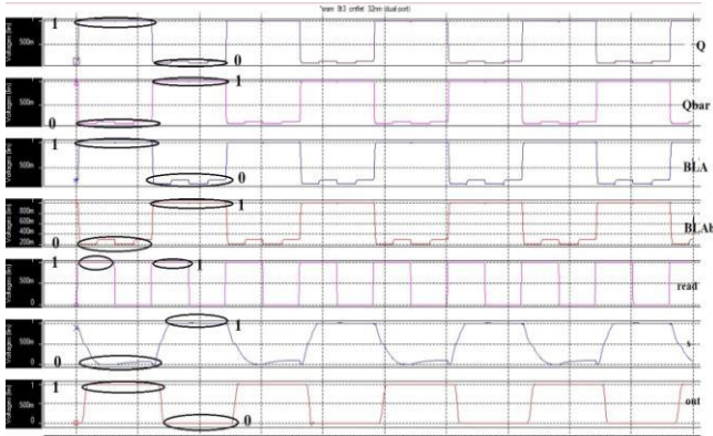
Fig. 7. Reading data from Dual-Port 8T CNTFET SRAM Cell Structure using bit lines (BLA & BLAb).
