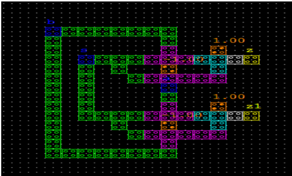
Fig.17 QCA layout for Proposed crossbar switch
