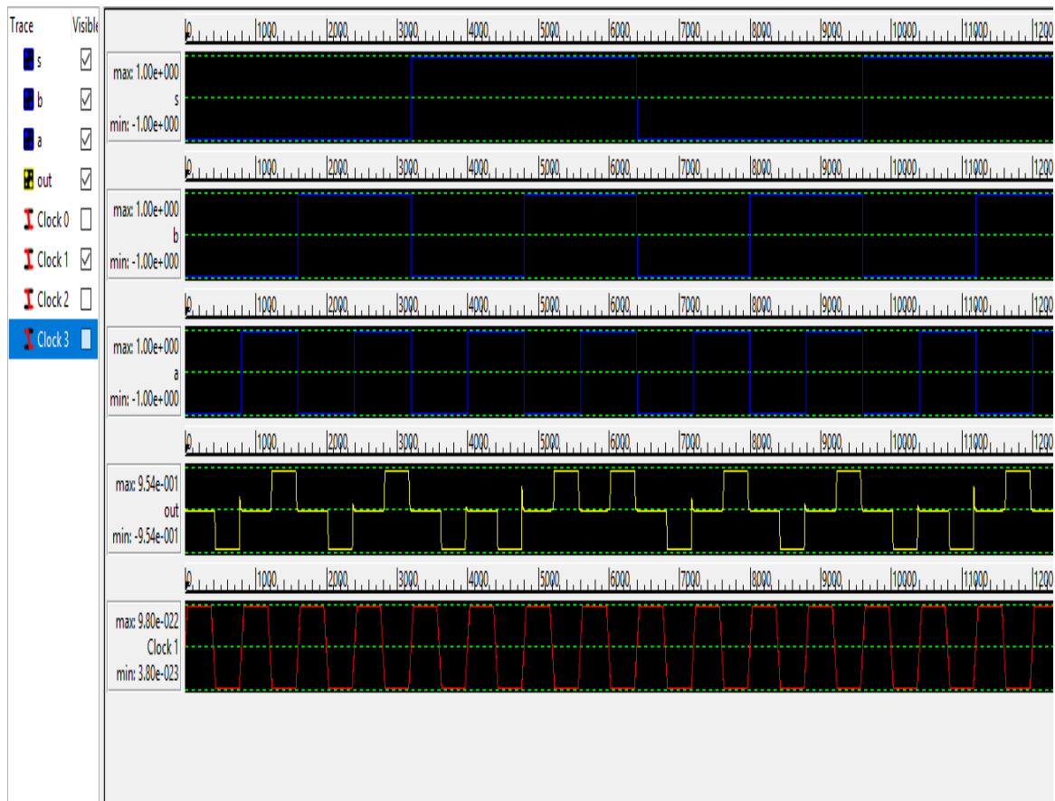
Fig.16 Simulation result for proposed 2x1 Multiplexer
