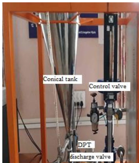
Figure 3 Real time conical tank system
