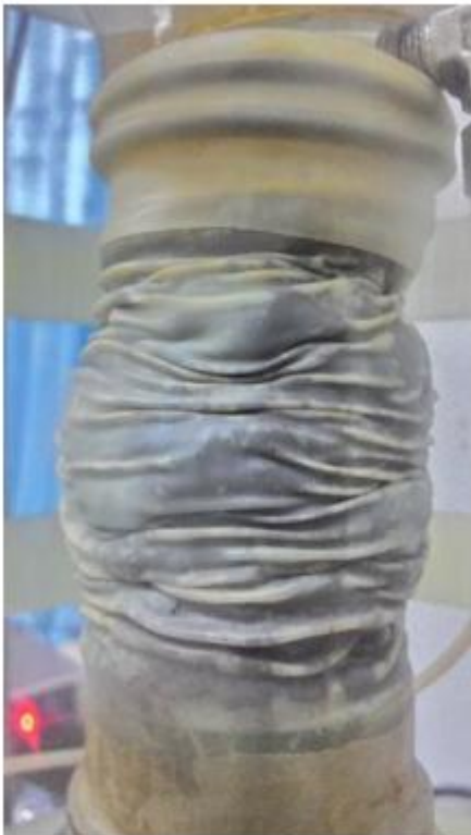
(b) PNpt-100 kPa-1.0Hz after Shearing Fig. 4. Failure Condition of Peat Soil.
