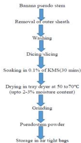
Fig.1 Flow chart for the preparation of Pseudostem powder
