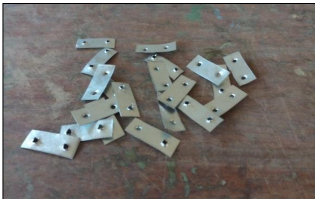
Fig. 2. Galvanized iron sheet placed between rubber.
