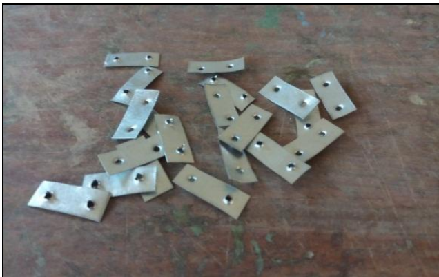
Fig. 2. Galvanized iron sheet placed between rubber.
